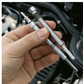
The reamer loosens coking that might occur after “baking-on” between glow plug and cylinder head.
