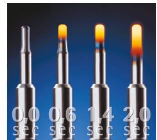
The BorgWarner Instant Start System enables key-turn start for compression-ignition engines just like that for a spark ignition engine.
