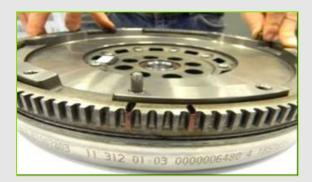
3. Mark the secondary flywheel position compared to the primary
