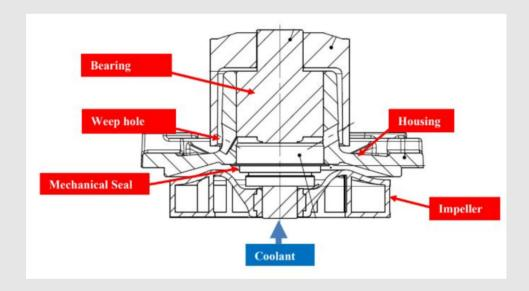
It is strongly recommended that before fitting a new water pump it is necessary not only to change the coolant, but also to clean the cooling circuit, otherwise when the pump starts to work again the coolant moves the residues / dirt around the cooling circuit causing the leakage through the mechanical seal and the pump's failure.
