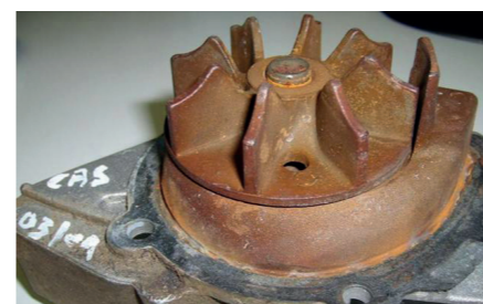
Figure 3: Corrosion in cooling system
